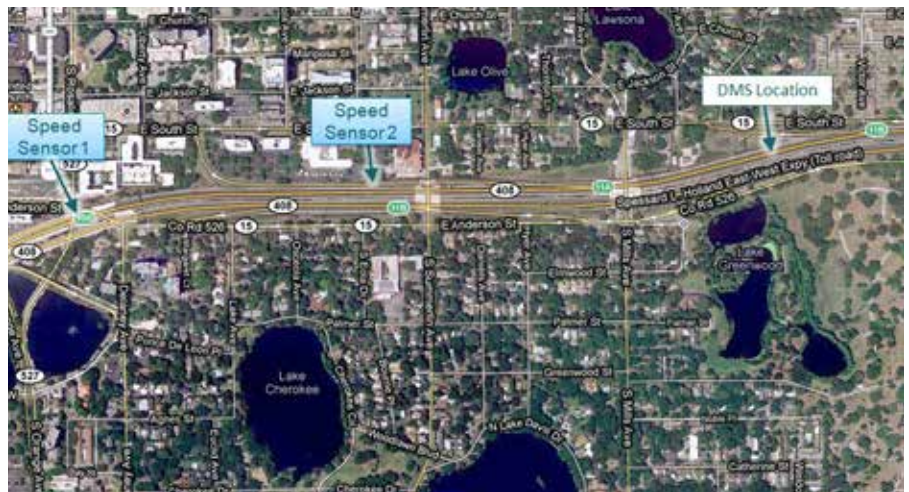
Figure 6. DMS and sensor locations for congestion alert system
