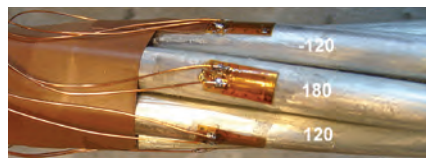
Figure 6. Strain gauges on three bottom wires of the strand
