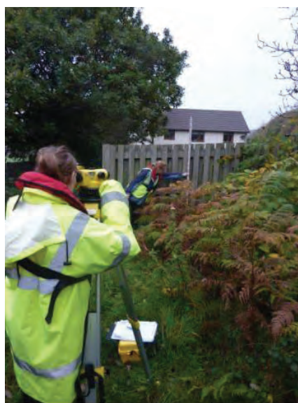
Figure 2. Measurement of river bed profile near Port Talbot, Wales leading to refinement of gradient effecting sediment deposition in HAWRAT
