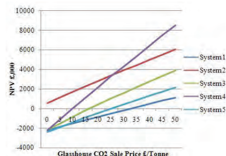
Figure 6. Effects on NPV due to variation in glasshouse CO 2 sale price with CO 2 recovery equipment investment at £1,000 k/MW e
