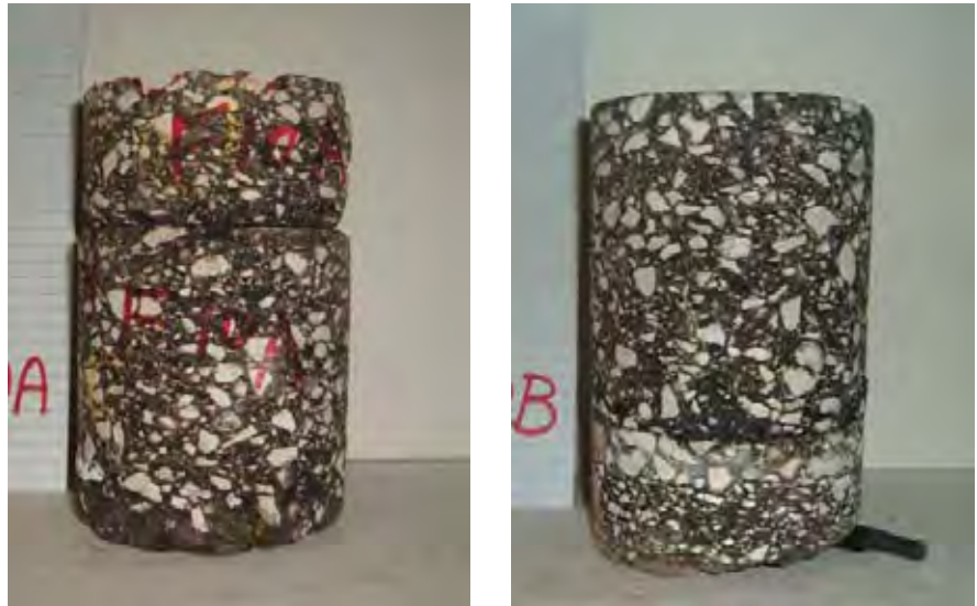
Figure 5. Representative core samples (F10A and F10B) showing air void and crack distributions in runway core samples
