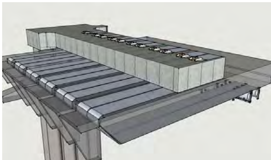
Figure 10. Anti-drag system with anchored steel sheets
