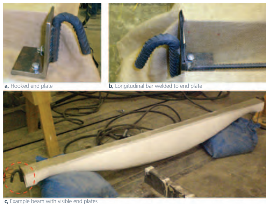
Figure 3. Anchorage using welded end plates
