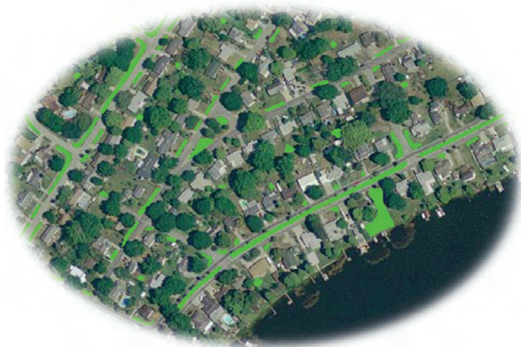
Figure 6 - Aerial photo of a residential neighborhood in southwest Winter Haven, showing a stormwater capture system that covers 5% of the surface area (highlighted in green). Source: Mark T. Brown for Atkins
