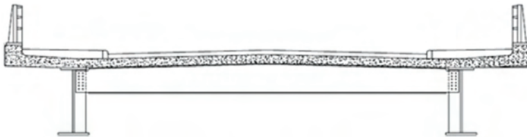
Figure 2 - Ladder deck bridge - typical cross section
