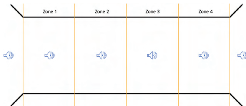
Figure 3 - A simplified layout of four tunnel zones that align with the fire ventilation plans plus one zone on each approach.
