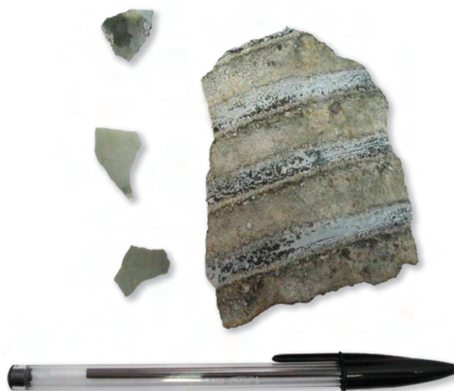
Figure 4 - Vivianite scale collected from the APD heat exchangers. The face showing is smooth and convex, the side attached to the corrugated tube of the heat exchanger. The concave side of the scale is exposed to the flow of sludge and is typically fibrous and rough. The three small samples to the left are calcite and were found adjacent to the heating elements, they are not thought to significantly impede heat transfer. Biro for scale.
