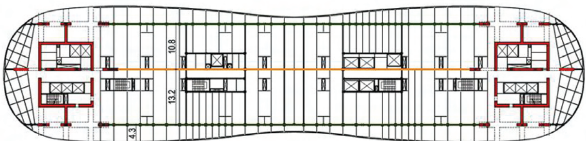
Figure 2 - Structural floor plan at level 34-Red: Main core walls and adjacent columns, Green: Outer wheel shape mega frame, Orange: Central wheel shape mega frame
