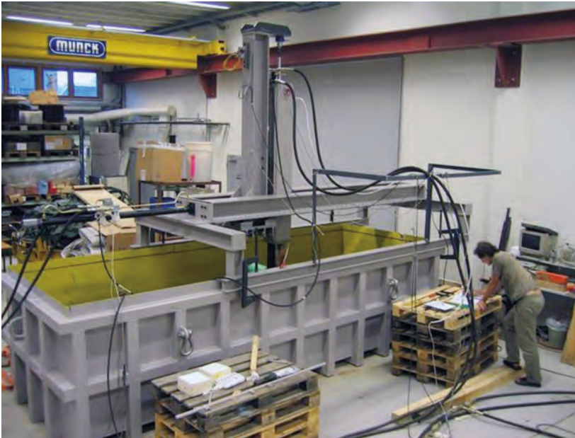
Figure 7 - Large-scale axial and lateral cyclic tests at NGI
