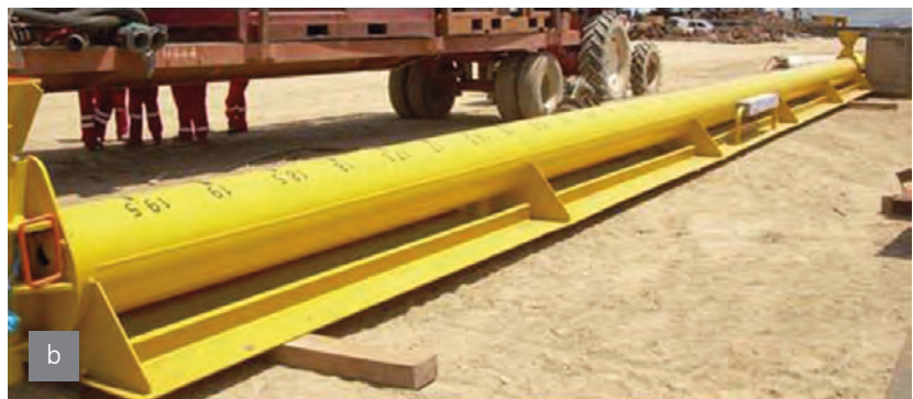
Figure 11 - Sleeper location plan (a) and sleeper assembly (b)
