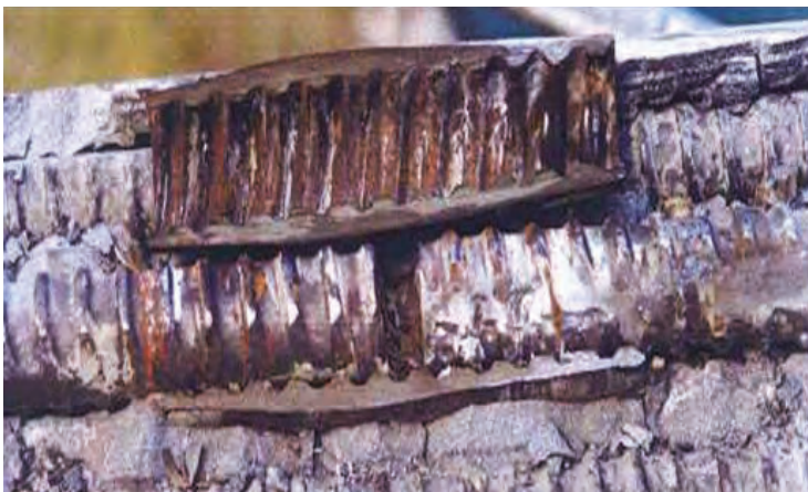
Figure 12 - Broken reinforcement coupler due to fatigue
