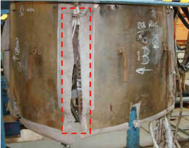
Figure 8 - Gap between the test chamber doors
