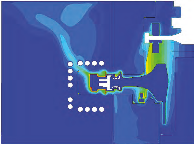
Figure 13 - Contours of velocity magnitude (m/s) (3D Sector)
