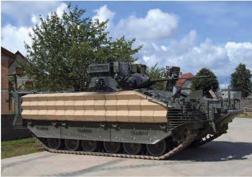
Figure 4 – Warrior armoured vehicle fitted with a mixture of bar armour and ERA
