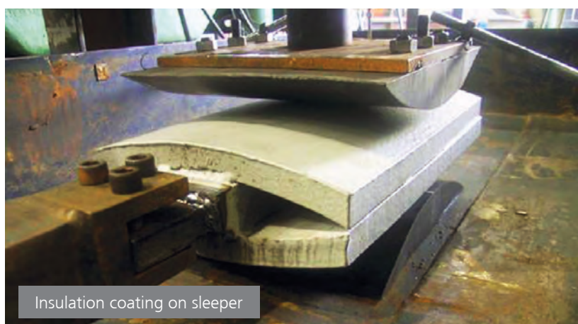
Figure 16 - Back-to-back pipe-sleeper test arrangement prior to seawater submersion
