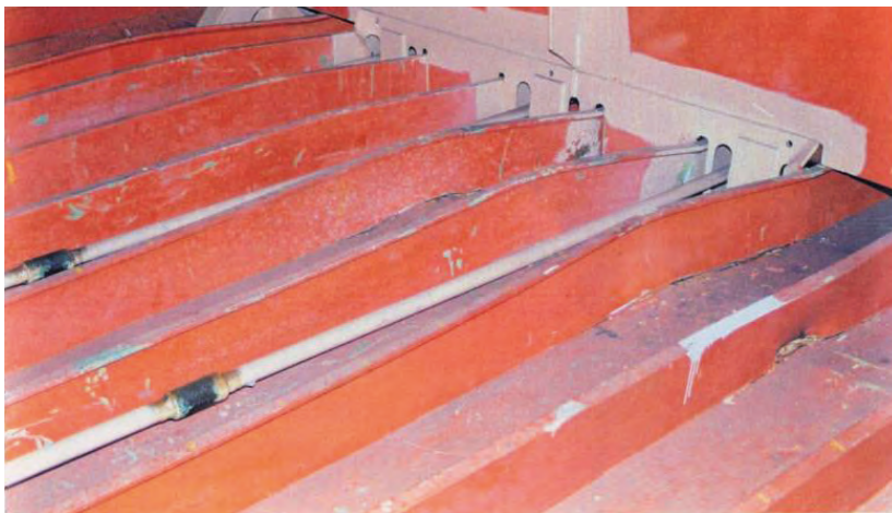
Figure 2 - Imperfections in longitudinal stiffeners following an impact
