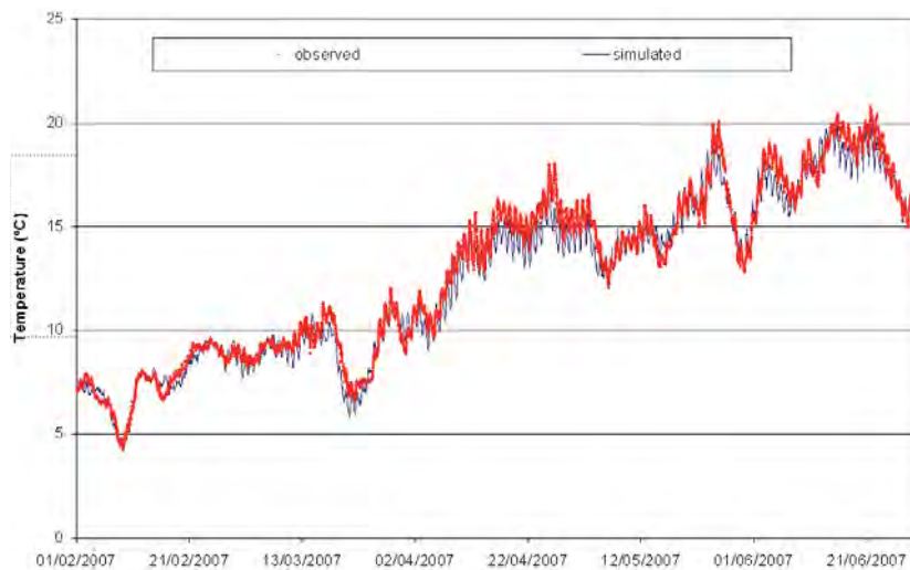
Figure 3 - Observed and simulated temperature at Plucks Gutter (15-min data; full calibration period).
