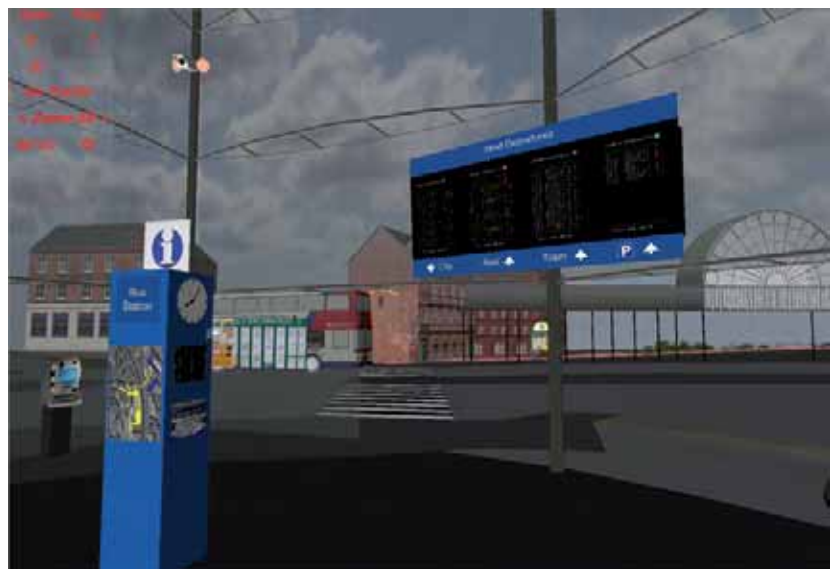
Figure 2 - During the construction of the model it was possible for the clients to compare LED (left) with Plasma (right) types of information displays
