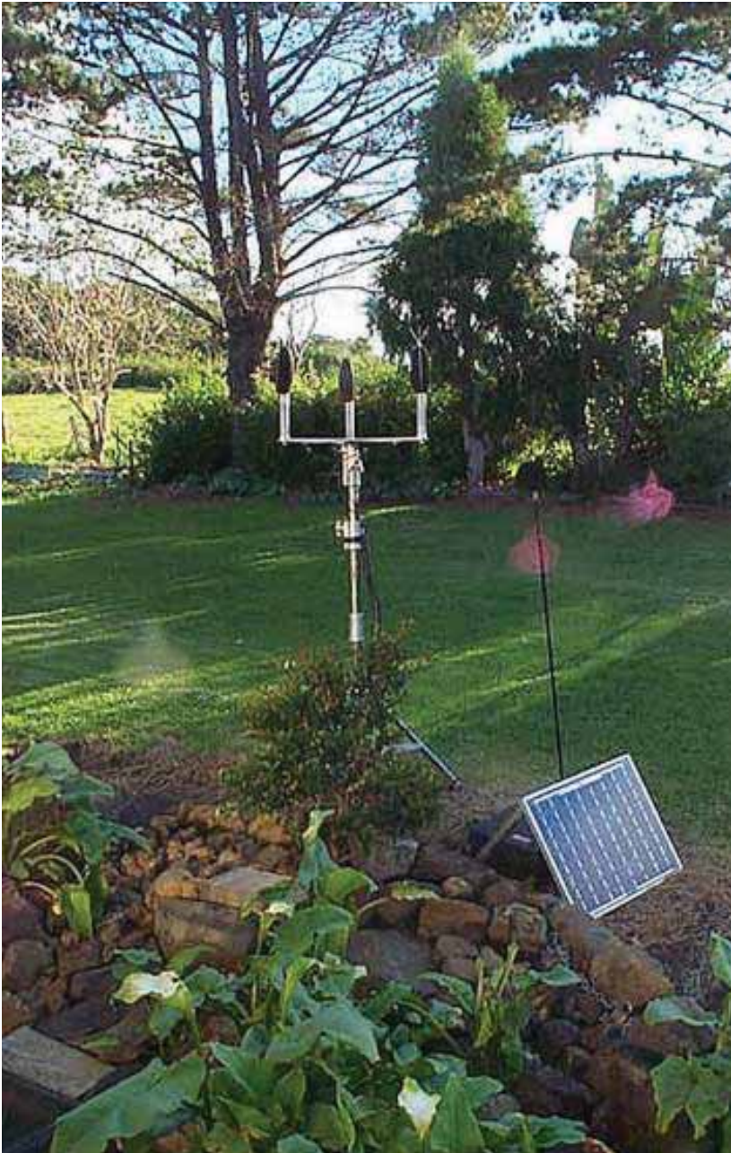
Figure 5 - Microphone array for directional monitoring
