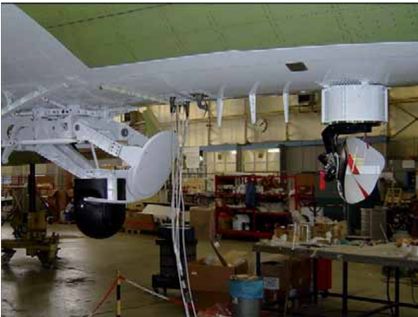
Figure 15 - FLIR Turret Assembly installed onto aircraft undergoing testing
