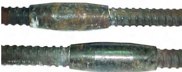
FIGURE 6. TYPICAL COUPLERS AND DIA- GRAMMATIC VIEW OF RESIN INJECTION
