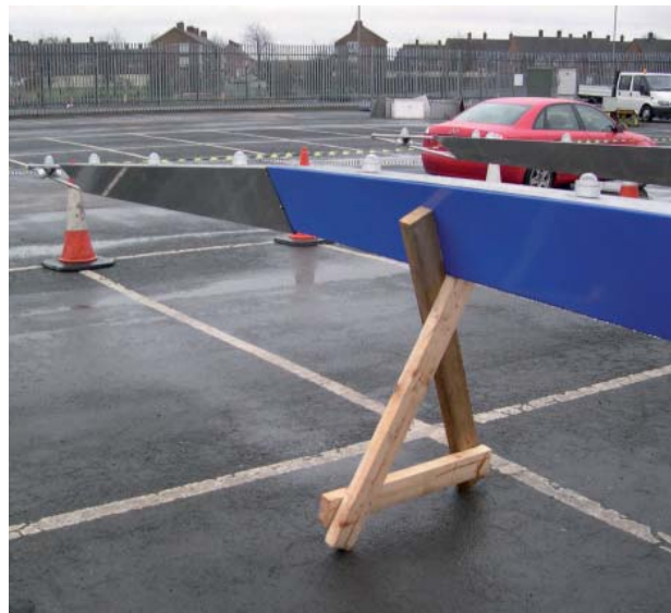
FIGURE 7. PERMANENT DEFORMATION IN MAST DUE TO GALLOPING
