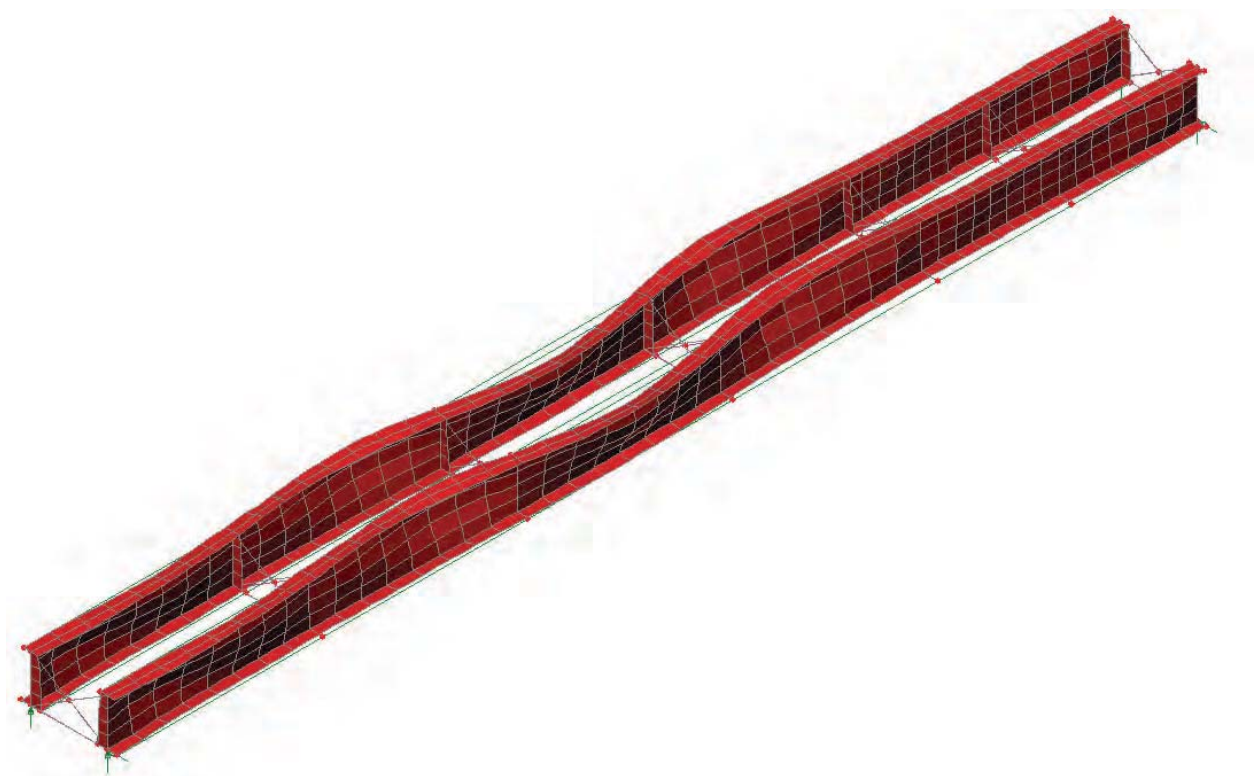
FIGURE 13. SECOND LOWEST GLOBAL MODE OF BUCKLING FOR SINGLE SPAN BEAMS
