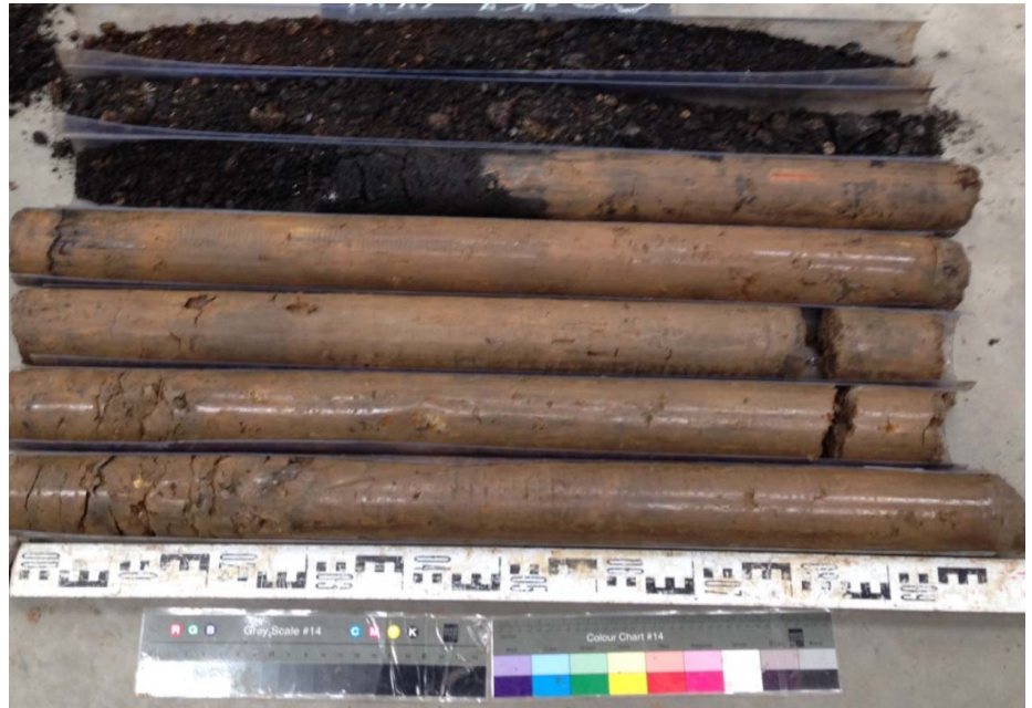
A) Ash and clinker overlying cohesive embankment fill in upper slope
