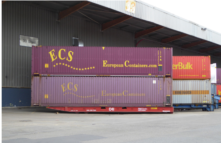
A) 45' containers on rolltrailers (note extensions of containers)
