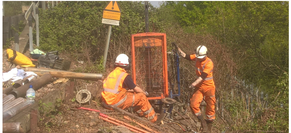
A) LLAMAR Rig set up at embankment crest at Country end of site for window sampling.
