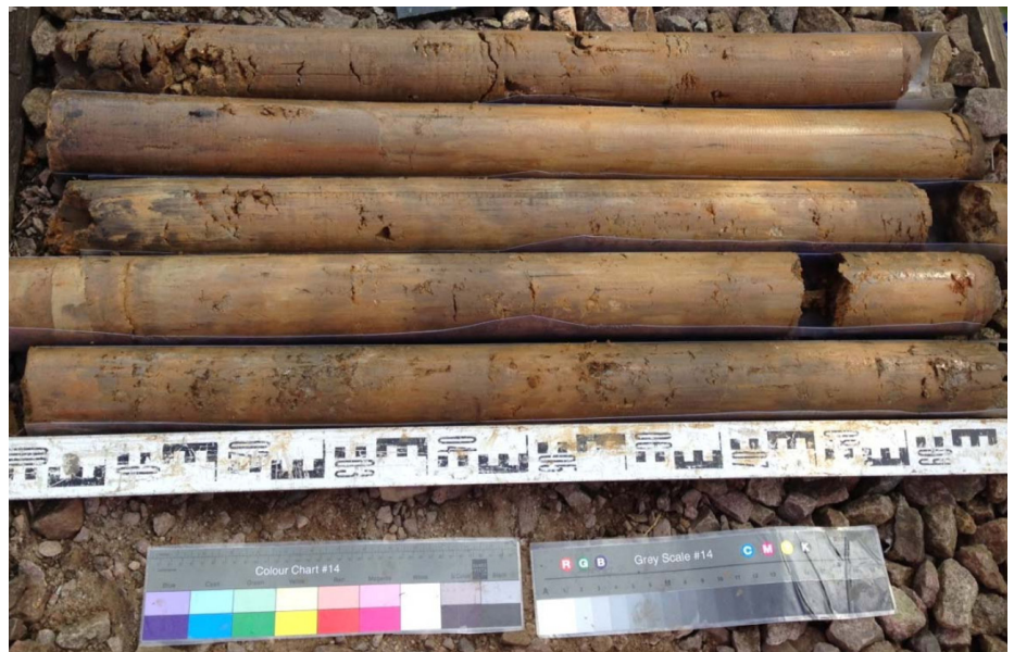
B) Absence of ash and clinker in lower slope.
