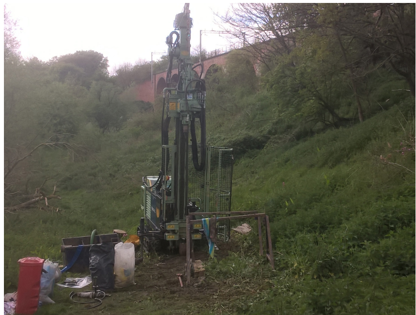
B) Rotary rig set up at embankment toe at London end of site for continuous sampling
