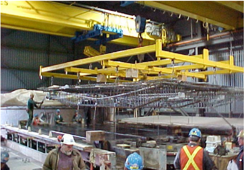
Pre-assembled Reinforcing Steel Cages
