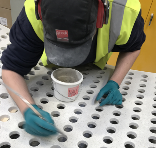
Figure 1: Production of acoustic GFRC panels at the GRCUK factory © GRCUK
