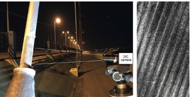
Figure 12: Daytime DIC measurement with unrestricted traffic and night measurement with 11 T vehicle
