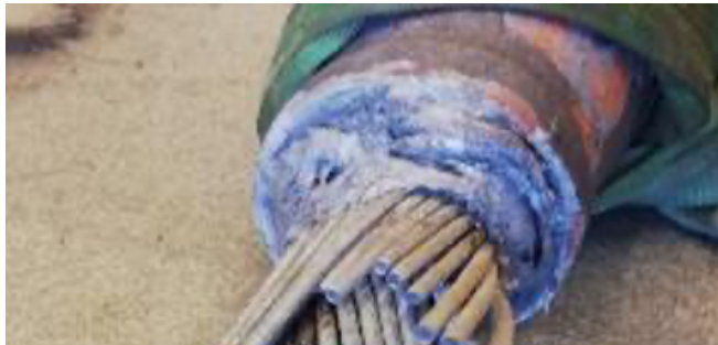
Figure 21: Tensile test failure in hanger 16-17 (other hanger failures similar)
