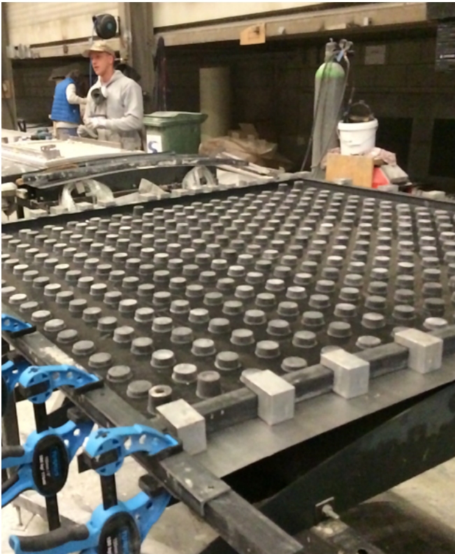
Figure 6: Deformable steel moulds at Concrete Valley © Sorba
