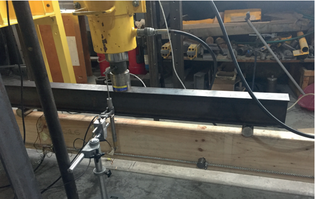
Figure 12: Testing for four-point bending tests.
