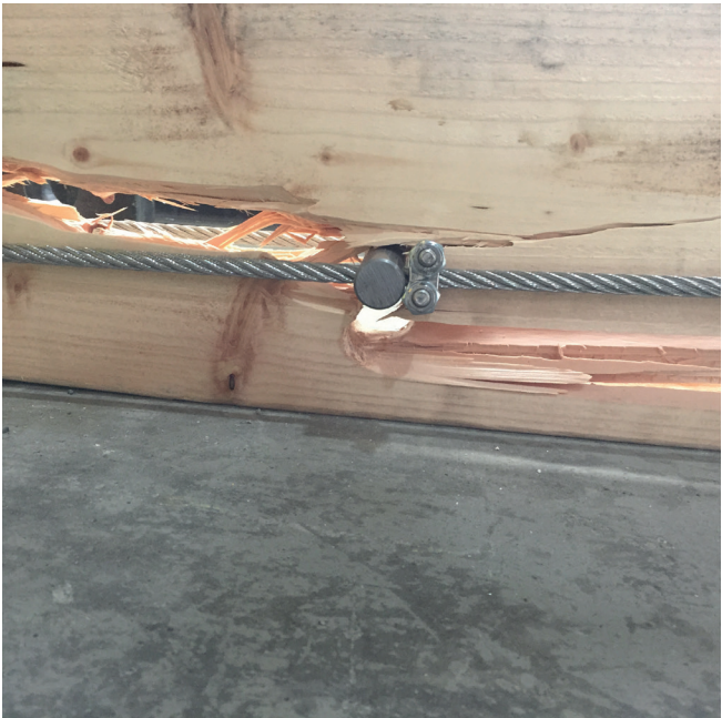
Figure 15: Tension crack around 25 mm ø spigot
