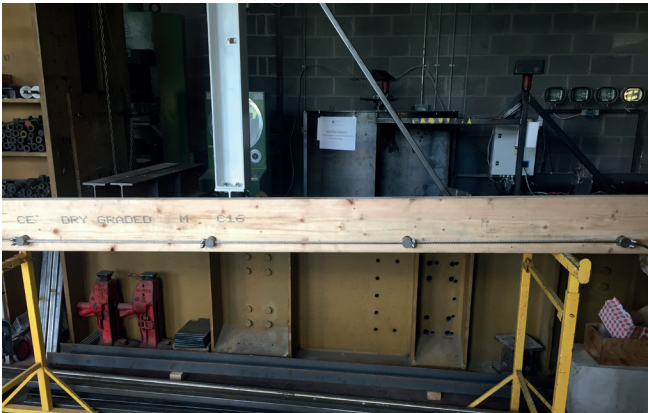
Figure 11: Reinforced timber beams with 4 no. 38 mm ø spigots
