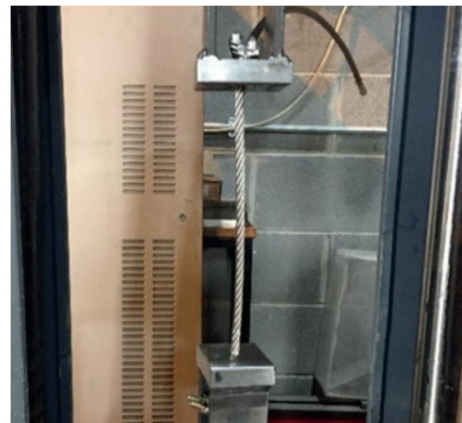
Figure 5: Image of cable and D clamp testing rig
