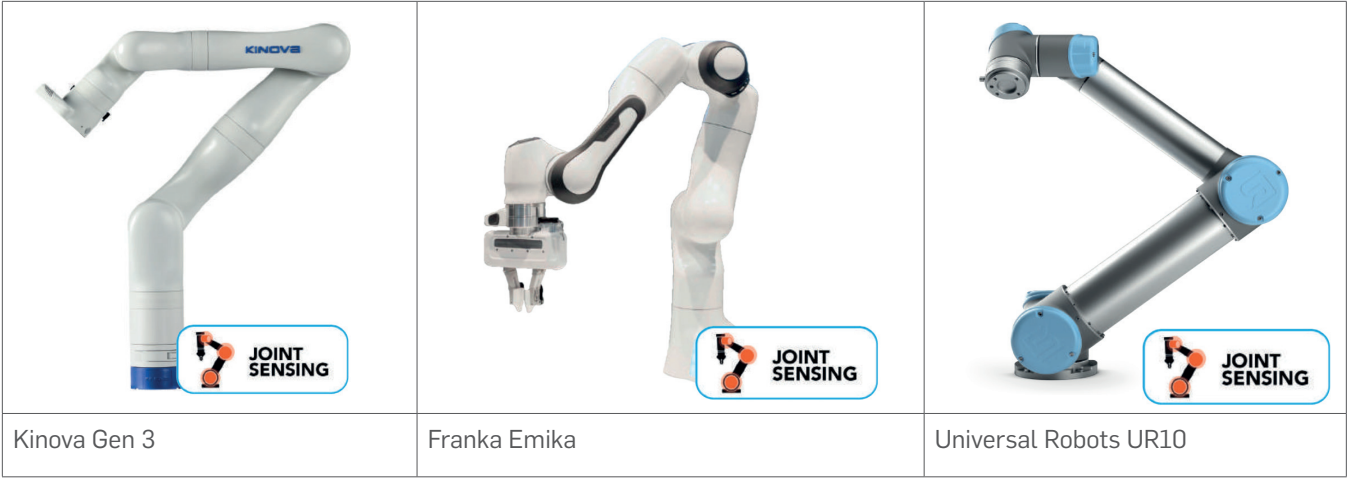
Figure 3: Three typical Cobot arms (Robotiq, 2020)
