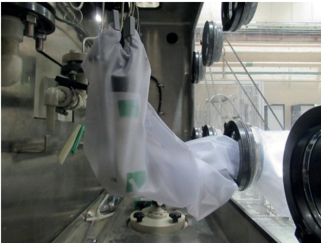
Figure 6b: Deployment system inside the glovebox in the inactive training facility
