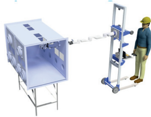
Figure 5: (a) Mobile deployment system outside of the glovebox (b) inserted in glovebox
