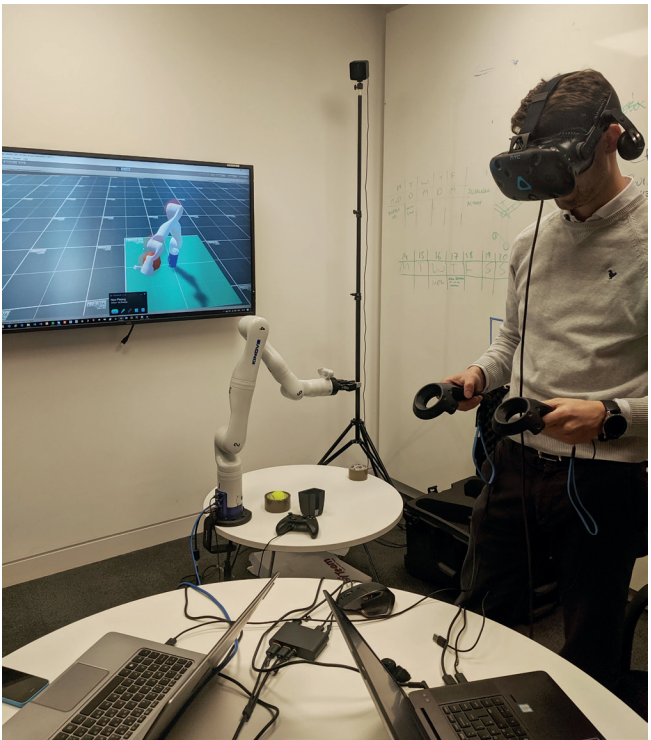
Figure 11: Virtual reality operation of the digital twin using the HTC Vive
