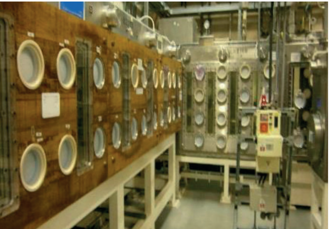
Figure 1: Typical glovebox train / wall configuration (FIS360, 2018)
