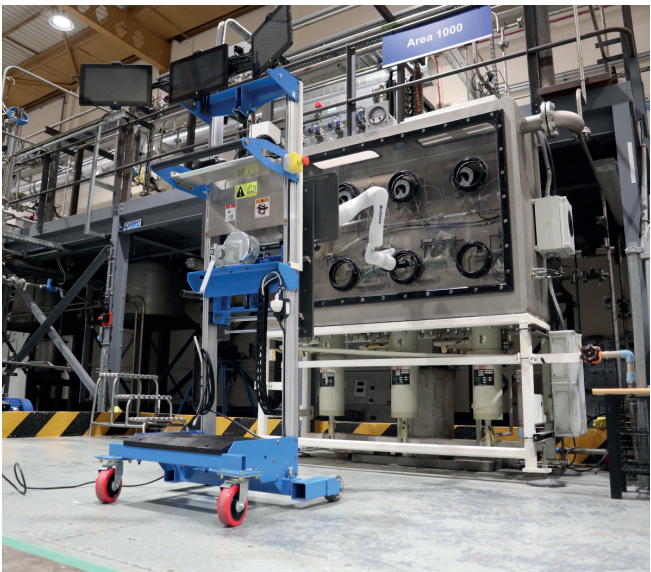
Figure 6a: Deployment system outside the glovebox in the inactive training facility
