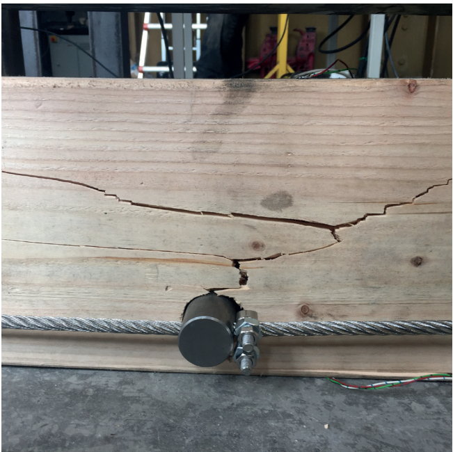
Figure 14: Tension crack around 38 mm ø spigot
