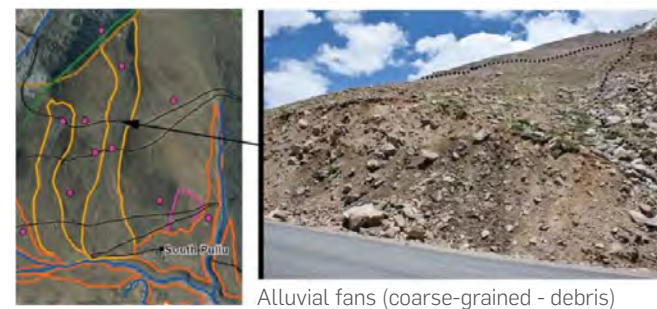
Figure 8: Debris Fans Mapped From Satellite Imagery and Confirmed by Ground Truthing.
